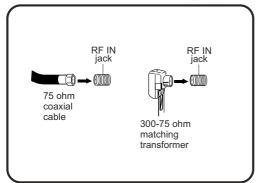
Connect the 75 ohm cable from the combination VHF/UHF antenna to the RF IN jack.
